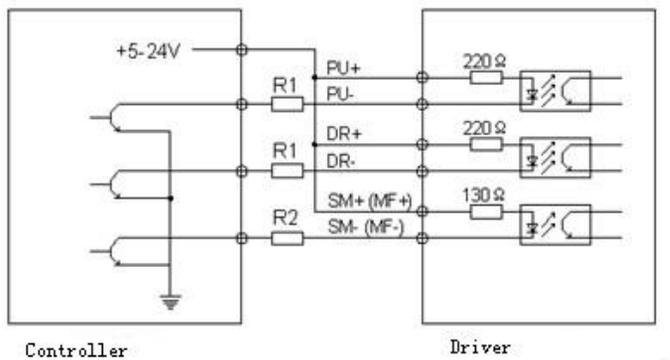
**Common Cathode Connection for Signal Input**
